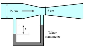
**Solution** A Venturi meter equipped with a water manometer is used to measure to flow rate of air through a duct. For a specified maximum differential height for the manometer, the maximum mass flow rate of air that can be measured is to be determined.
