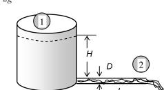
Solution A water tank open to the atmosphere is initially filled with water. The tank is drained to the atmosphere through a 90° horizontal bend of negligible length. The flow rate is to be determined for the cases of the bend being a flanged smooth bend and a miter bend without vanes.
