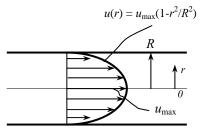
**Discussion** A unique feature of fully developed laminar pipe flow is that the maximum velocity is exactly twice the average velocity. This is *not* the case for turbulent pipe flow, since the velocity profile is much fuller.
