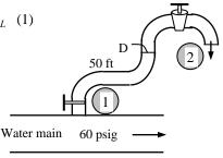
**Solution** A water fountain is to be installed at a remote location by attaching a cast iron pipe directly to a water main. For a specified flow rate, the minimum diameter of the piping system is to be determined.
