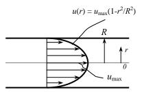
*Discussion* Compared to the previous problem, the average velocity remains the same since the maximum velocity (at the centerline) remains the same, but the volume flow rate increases as the diameter increases.
