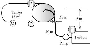
which is greater than 4000. Therefore, the flow is turbulent. The friction factor can be determined from the Moody chart, but to avoid the reading error, we determine it from the Colebrook equation,
