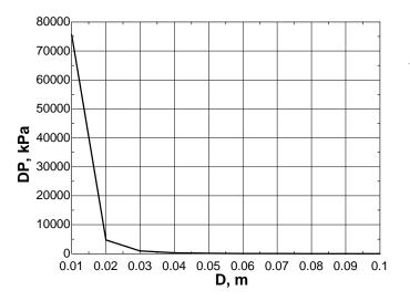
*Discussion* The pressure drop decays quite rapidly with increasing diameter – by several orders of magnitude, in fact. We conclude that larger diameter pipes are better when pressure drop is of concern. Of course, bigger pipes cost more and take up more space, so there is typically an optimum pipe size that is a compromise between cost and practicality.
