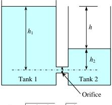
$$\frac{P_1}{\rho g} + \frac{V_1^2}{2g} + z_1 = \frac{P_0}{\rho g} + \frac{V_0^2}{2g} + z_0 \rightarrow \frac{P_{atm}}{\rho g} + h_1 = \frac{P_{atm} + \rho g h_2}{\rho g} + \frac{V_0^2}{2g} \rightarrow V_0 = \sqrt{2g(h_1 - h_2)} = \sqrt{2gh}$$
