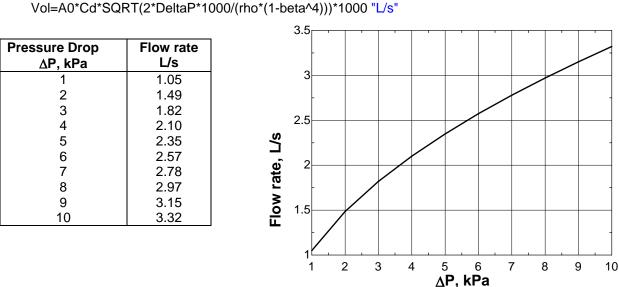
*Discussion* This type of plot can be thought of as a calibration plot for the flowmeter, although a real calibration plot would use actual experimental data rather than data from equations. It would be interesting to compare the above plot to experimental data to see how close the predictions are.
