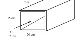
The friction factor can be determined from the Moody chart, but to avoid the reading error, we determine it from the Colebrook equation using an equation solver (or an iterative scheme),
