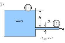
**Solution** A horizontal water pipe has an abrupt expansion. The water velocity and pressure in the smaller diameter pipe are given. The pressure after the expansion and the error that would have occurred if the Bernoulli Equation had been used are to be determined.
