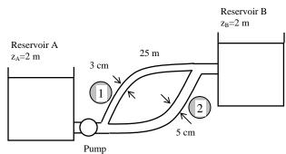
*Analysis* This problem cannot be solved directly since the velocities (or flow rates) in the pipes are not known. Therefore, we would normally use a trial-and-error approach here. However, nowadays the equation solvers such as EES are widely available, and thus below we will simply set up the equations to be solved by an equation solver. The head supplied by the pump to the fluid is determined from
