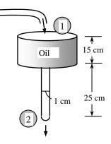
which is less than 2300. Therefore, the flow is laminar, as postulated. (Note that in the actual case the velocity and thus the Reynolds number will be even smaller, verifying the flow is always laminar). The entry length in this case is
