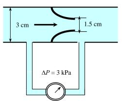
which is equivalent to 0.429 L/s. The average flow velocity in the pipe is determined by dividing the flow rate by the cross-sectional area of the pipe,
