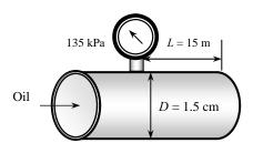
**Solution** Glycerin is flowing through a horizontal pipe which discharges into the atmosphere at a specified flow rate. The absolute pressure at a specified location in the pipe, and the angle  $\theta$  that the pipe must be inclined downwards for the pressure in the entire pipe to be atmospheric pressure are to be determined.
