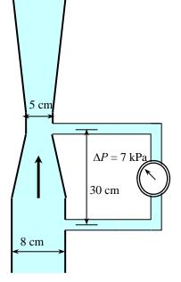
*Discussion* Note that the elevation difference between the locations of the two probes does not enter the analysis since the pressure gage measures the pressure differential at a specified location. When there is no flow through the Venturi meter, for example, the pressure gage would read zero.
