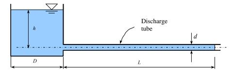
*Assumptions* 1 The fluid is incompressible. 2 The discharge tube is horizontal, and the flow is laminar. 3 Entrance effects and the velocity heads are negligible.
