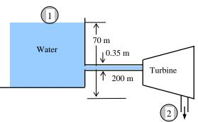
**Solution** In a hydroelectric power plant, the flow rate of water, the available elevation head, and the combined turbine-generator efficiency are given. The percent increase in the electric power output of the plant is to be determined when the pipe diameter is tripled.
