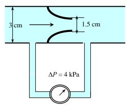
which is equivalent to 0.627 L/s. The average flow velocity in the pipe is determined by dividing the flow rate by the crosssectional area of the pipe,
