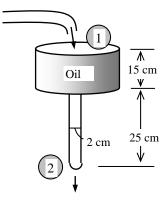
which is less than 2300. Therefore, the flow is laminar. (Note that in the actual case the velocity and thus the Reynolds number will be even smaller, verifying the flow is always laminar). The entry length is
