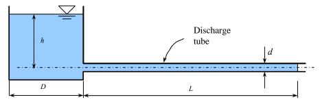
Assumptions 1 The oil is incompressible. 2 The discharge tube is horizontal, and the flow is laminar. 3 Entrance effects and the inlet and the exit velocity heads are negligible.
