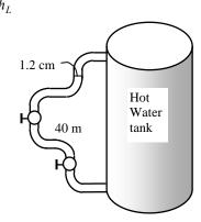
which is greater than 4000. Therefore, the flow is turbulent. The friction factor corresponding to the relative roughness of zero and this Reynolds number can simply be determined from the Moody chart. To avoid the reading error, we determine it from the Colebrook equation,
