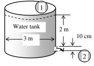
The average discharge velocity through the orifice at any given time, in general, can be expressed as
