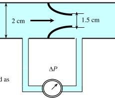
**Solution** The flow rate of water is to be measured with flow nozzle equipped with an inverted air-water manometer. For a given differential height, the flow rate and head loss caused by the nozzle meter are to be determined.
