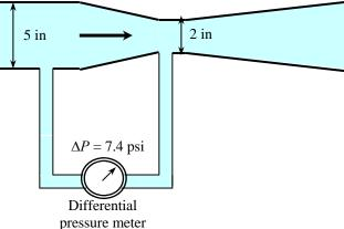
Also, the average flow velocity in the pipe is determined by dividing the flow rate by the cross-sectional area of the pipe,
