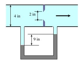
**Solution** The flow rate of water is measured with an orifice meter. The pressure difference indicated by the orifice meter and the head loss are to be determined.
