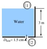
Solution Water is discharged from a water reservoir through a circular hole of diameter D at the side wall at a vertical distance H from the free surface. A relation for the "equivalent diameter" of the sharp-edged hole for use in frictionless flow relations is to be obtained.
