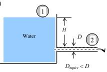
Discussion Note that the effect of frictional losses of a sharp-edged entrance is to reduce the diameter by about 10%. Also, noting that the flow rate is proportional to the square of the diameter, we have  $\dot{V} \propto D_{equiv}^2 = (0.904D)^2 = 0.82D^2$ . Therefore, the flow rate through a sharp-edged entrance is about 18% less compared to the frictionless entrance case.
