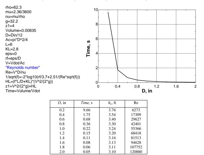
Discussion The required time decreases considerably as the tube diameter increases. This is because the irreversible frictional head loss (major loss) in the tube decreases greatly as tube diameter increases. In addition, the minor loss is proportional to  $V^2$ . Thus, as tube diameter increases, V decreases, and even the minor losses decrease.
