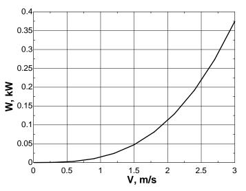
*Discussion* As you might have suspected, the required power does not increase linearly with average velocity. Rather, the relationship is nearly quadratic. A larger diameter pipe would cut reduce the required pumping power considerably.
