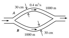
**Solution** Cast iron piping of a water distribution system involves a parallel section with identical diameters but different lengths and different valves. The flow rate through one of the pipes is given, and the flow rate through the other pipe is to be determined.
